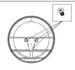
4. Remove the screw connecting the cabinet to the door .
